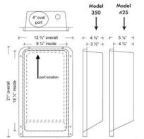
For Upward Exhaust Direction
